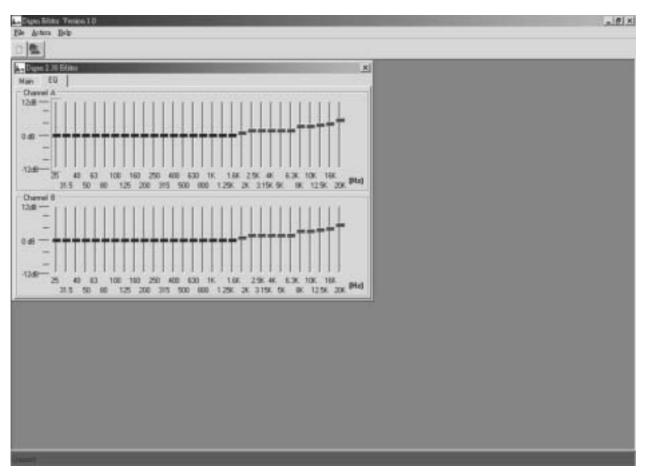
When you go to the EQ menu, the PC will display above picture. You can adjust each band's gain value, if this unit is in LINK function, the change on channel A will be applied to channel B also. The adjustable range goes from 12dB to +12dB.
