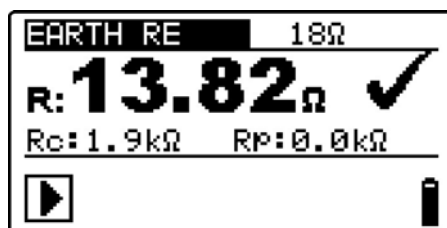
Figure 5.35: Example of earth resistance measurement result
