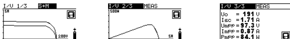
Figure 6.21: Example of I / V curve results
