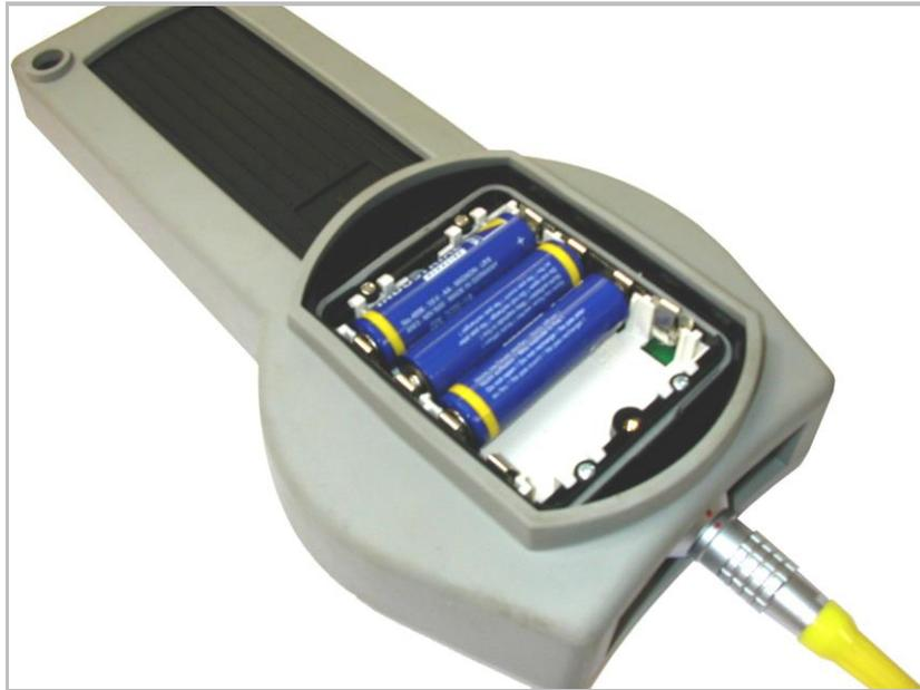
**Battery compartment & flylead socket**
