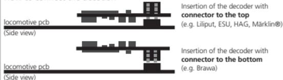
Figure 3: LokPilot V4.0 (DCC) - 21MTC
