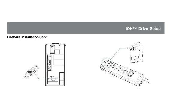
**Step 3.** Plug the FireWire 6 pin connector into your computer's FireWire Port.
