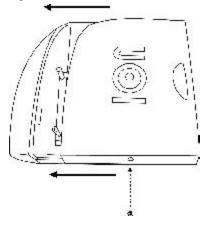
Step. 11 Place assembled enclosure back into the base.
