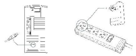
Step 3. Plug the USB Type A connector into your computer's USB 2.0 Port.
