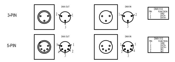
Connection between controller and projector and between one projector and another must be made with a 2 core-screened cable, with each core having at least a 0.5mm diameter. Connection to and from the projector is via cannon 5 pin (which are included with the projector) or 3 pin XLR plugs and sockets. The XLR's are connected as shown in the figure above.
