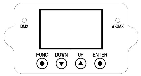
Projector configuration can be set conveniently via press button switch and LCD display.
