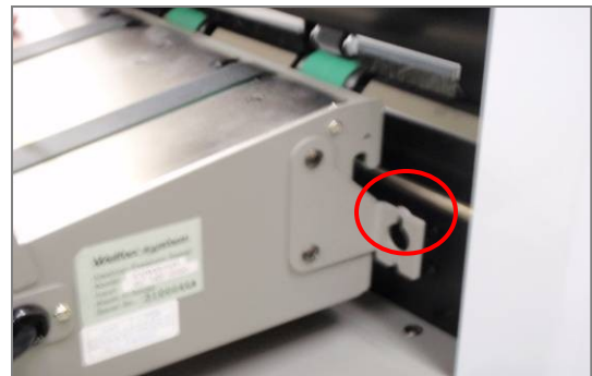
Place the conveyor on to IM-9500
