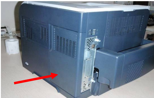
Remove this cover from the printer to access the communication part of printer
