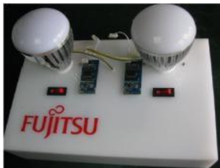
Figure 3-10: step 2-Install lighting bulb (completed)
