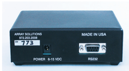
Photo 2: Rear panel connections for DC power and RS-232
