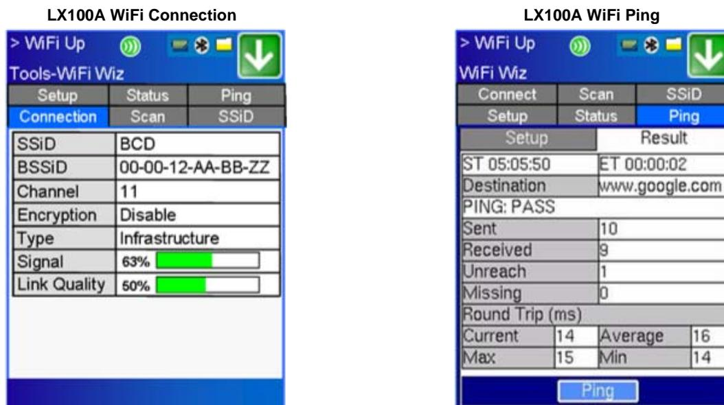
**Ping** - Before performing the Ping test, ensure the WiFi connection is Up and the WiFi icon (on the top of the screen) has turned green.
