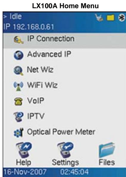
The upper part of the menu (IP connection, Advanced IP, Net Wiz, WiFi Wiz, VoIP, IPTV and Optical Power Meter) consists of applications specific to the test set, while the lower part of the menu contains applications (Help, Settings, Files) which are common to all VeEX VePAL handheld test sets.
