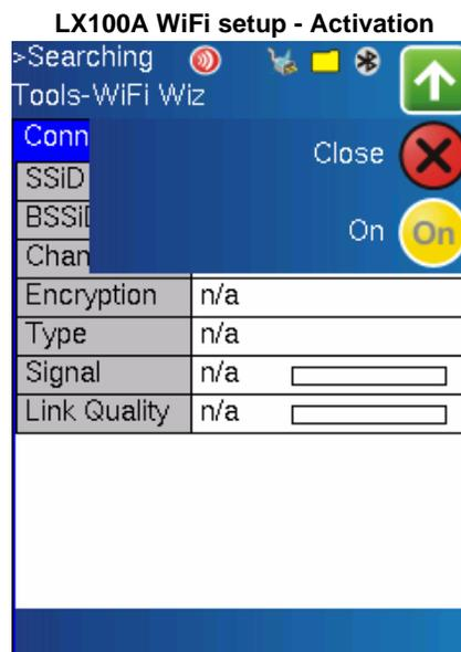
**Scan** - Tap on the Scan tab once the test set has detected the wireless USB adapter. Press Scan on the bottom to start scanning the site. When scan is completed, the test set will show the number of SSIDs, Channels, and the number of SSIDs in Infrastructures mode and Ad-Hoc mode.
