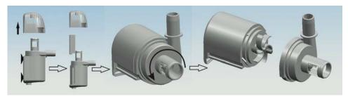
**Pump**: To prevent build up of sediment, scale or dirt in the impeller or filter, remove the pump cover and the impeller cover. Clean parts with a soft brush, and mild soap and water.
