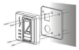
4) Use screws to fix the device and waterproof glue on the wall.
