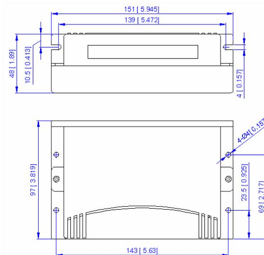
Figure 1: Mechanical specifications
