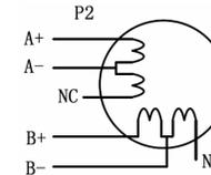
Figure 6: 6-lead motor half coil (higher speed) connections
