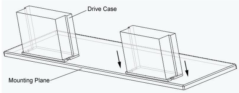
**Important NOTE:** The driver must be mounted vertically onto a plate or a heat sinking to maximize heat sink area as shown in the above picture. Please use additional heat sinking or cool fan if necessary.
