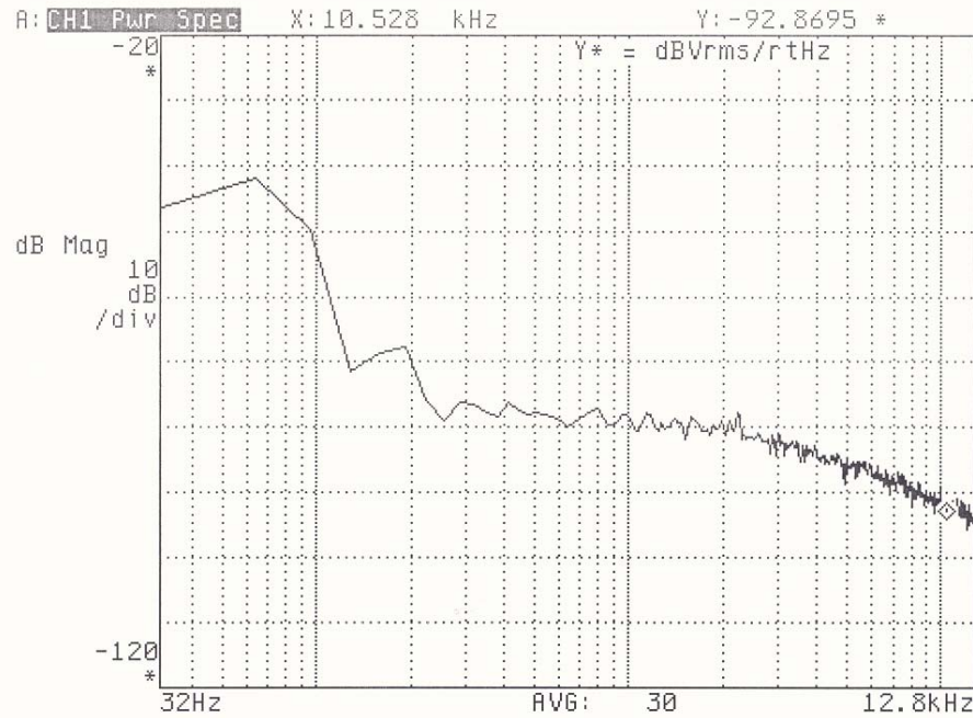
Figure 3-6 SQUID noise spectrum at (0-12.8 kHz), 81.8 Kelvin, gain=x100
