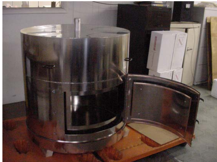
Figure 6-9 Option MS-770 two layer mu metal shield
