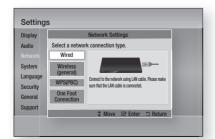
2 Press the **FNTFR** button The Network Status screen appears. The player connects to the network after the network connection is verified.
