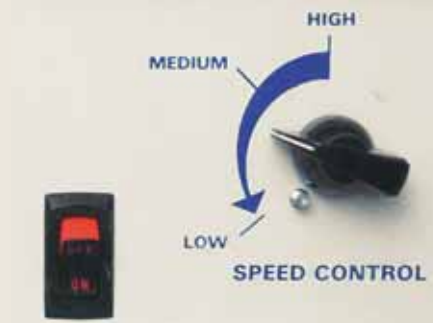
FIGURE 7 The flow rate on this machine is adjusted with the dial on the right-hand side.
