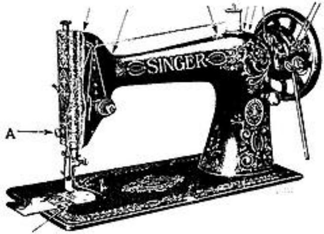
FIG. 17. FRONT VIEW, SHOWING OILING POINTS
