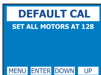
RESET EEPROM. RESET ALL SETTINGS TO 128 VALUE
