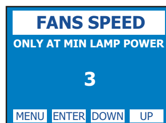
FAN SPEED WHEN DIMMER CLOSED
