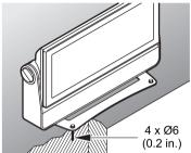
Two quarter-turn brackets are supplied with the device if it is to be flown above the ground. Remove the floor stand/base and rig the P-5 to a support truss or structure using the supplied brackets and suitable clamps.
