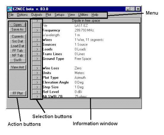
**Information Window** – This window shows information about a number of important parameters of the antenna being modeled. Any of the information in this window which can be changed is saved with the antenna description in the antenna description file.
