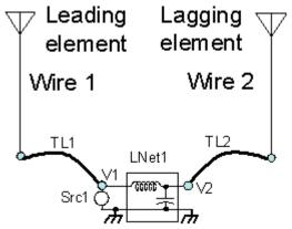
Of course, transmission lines TL1 and TL2 each have two conductors, and the models have two sets of two terminals just like the L network object LNet1. The second conductor is omitted from the diagram for simplicity.
