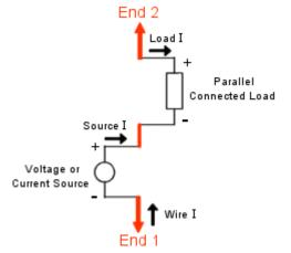
Compare this to the first diagram, with the series connected load, and it's apparent that the definitions of polarity of both the load voltage and current are opposite for the two types of loads. This has no impact on any results except for the phase angle of voltage and current shown in the Load Data display.
