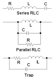
Values of R, L, and C are entered in the appropriate columns. **EZNEC** will calculate and use the impedance of the RLC combination as required.
