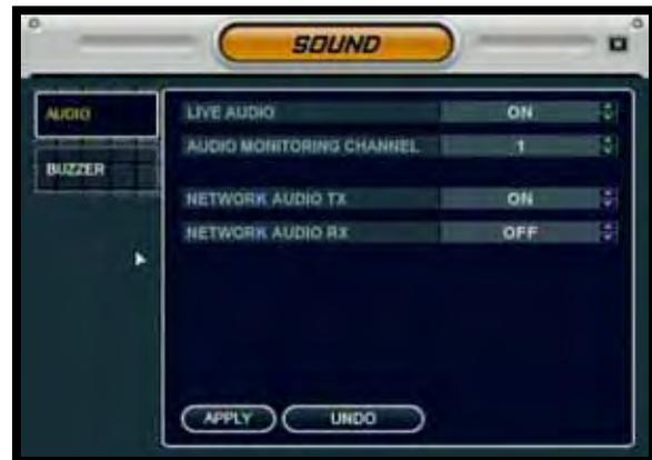
**NOTE:** Once the LIVE AUDIO Feature has been set to ON, the Remote Control can be used to select the Listen-In Audio Channel. Press the AUDIO button on the Remote Control to switch between Channels 1~4.
