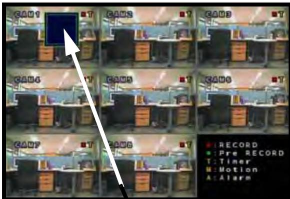
1. Press the ENTER button on the Remote. The Highlight will change to YELLOW - Setup Mode is now active.
