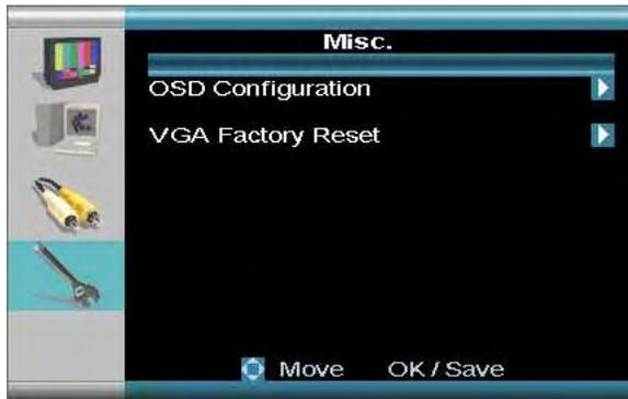
Use the Arrow keys on the front panel or remote control to access the OSD Configuration or VGA Factory Reset submenus. Change the values using the arrow keys and enter.
