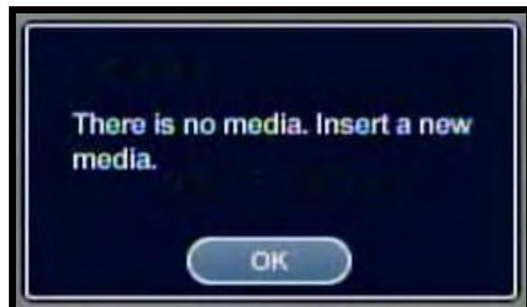
Error dialogue displayed when the backup device (USB) is not detected
