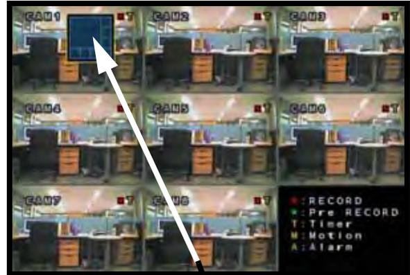
2. Select the Display Mode by pressing the Left and Right buttons (7 different Display Options - Single, Quad, 6-split, 8 split, 9-split, 13 split, 16 split).
