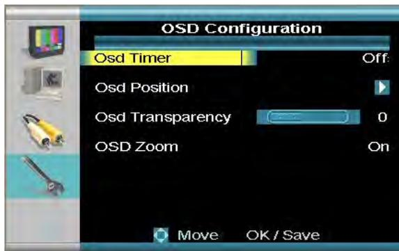
Use the Up, Down, Left and Right arrows to adjust the settings. Press the Enter button to set, and the Return button to exit the menu.
