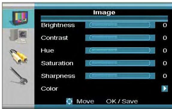
Use the Arrow keys on the front panel or Remote Control to select from Brightness, Contrast, Hue, Saturation, Sharpness or enter the Color submenu. Change the values using the arrow keys and enter.
