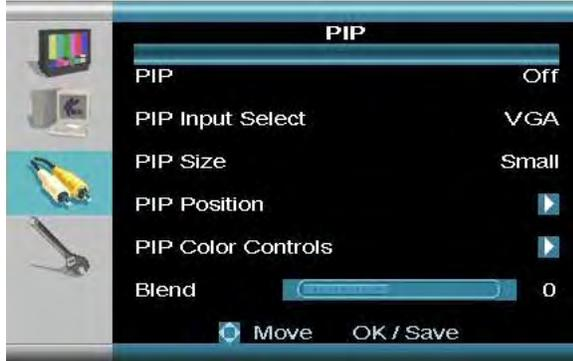
Use the Arrow keys on the front panel or remote control to select from PIP, PIP Input Select, PIP Size and Blend. Use the enter key to access the PIP Position or Pip Color Control submenus. Change the values using the arrow keys and enter.
