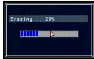
The Erasing status window displays the completion state of the Erasing of previously archived data (in%)
