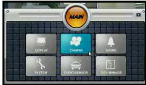
2. Select the CAMERA menu from the MAIN menu. Navigate using the up and down arrows on the front panel (or remote control). Highlight the selection in Green, and press the ENTER button to enter the CAMERA Menu.
