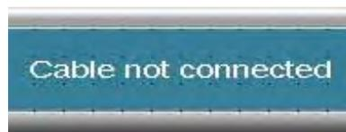
**Cable Not Connected:** Indicates that the VGA cable has not been securely fastened to either the system or PC.
