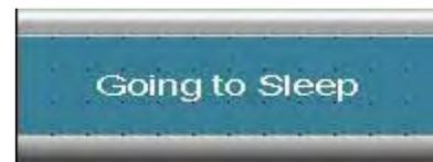
**Going to Sleep:** Indicates that the system is not receiving a signal from the PC, and is going into hibernation. This does not affect the DVR functions.
