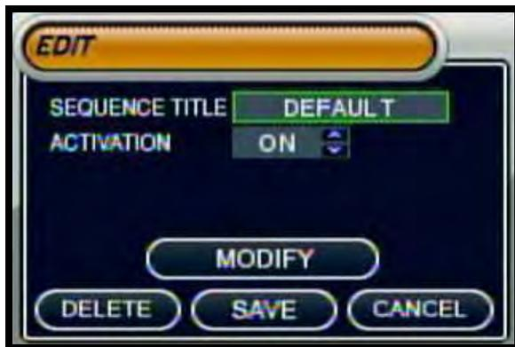
**NOTE:** The system will prompt you for "MOUSE OPERATION ONLY," however, you can modify the Sequence setup using the remote control.
