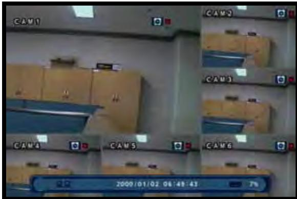
6. Press the SEQUENCE button on the Remote or Mouse Menu to switch to Sequence display.
