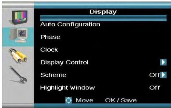
Use the Arrow keys on the front panel or Remote Control to select from Auto Configuration, Phase, Clock or Highlight Window. Use the enter key to access the Display Control or Scheme submenus. Change the values using the arrow keys and enter.
