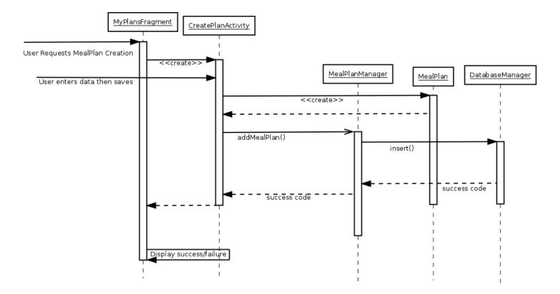
Sequence Diagram for Joining a Meal Plan
