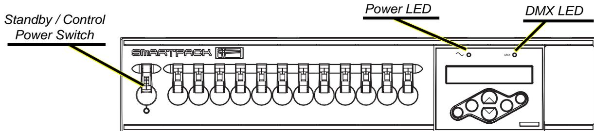
Use the Standby/Control power switch to start up and shut down operation of the SmartPack. When the breaker is in the ON position, the blue Power LED is illuminated indicating the power is on.
