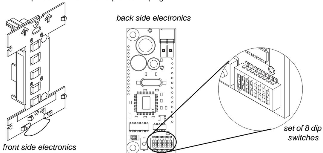
The table below indicates dip switch settings for both the 5 button and the 10 button preset stations.
