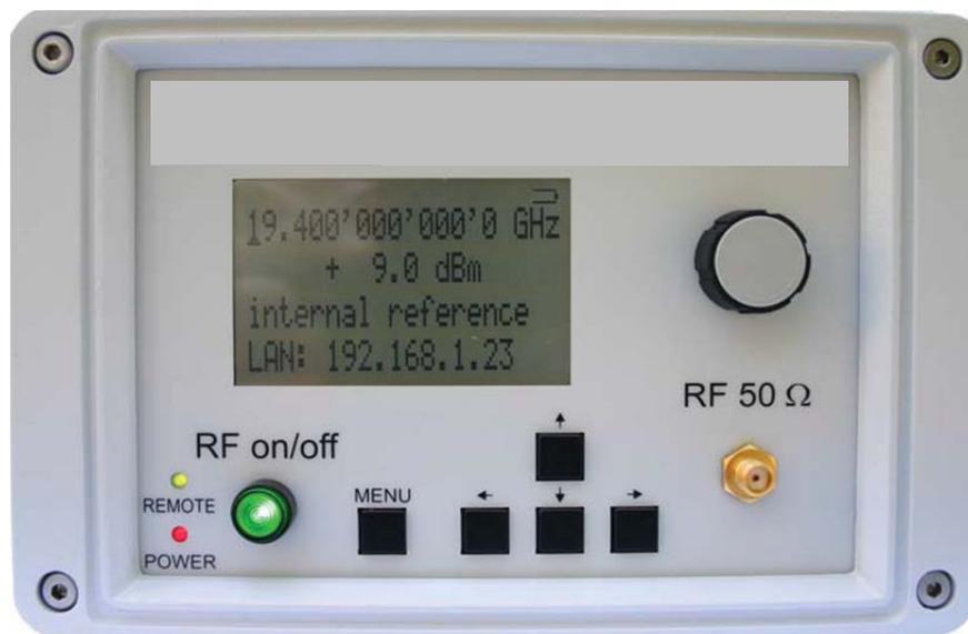
Figure 1 Front Panel View (835-3)
