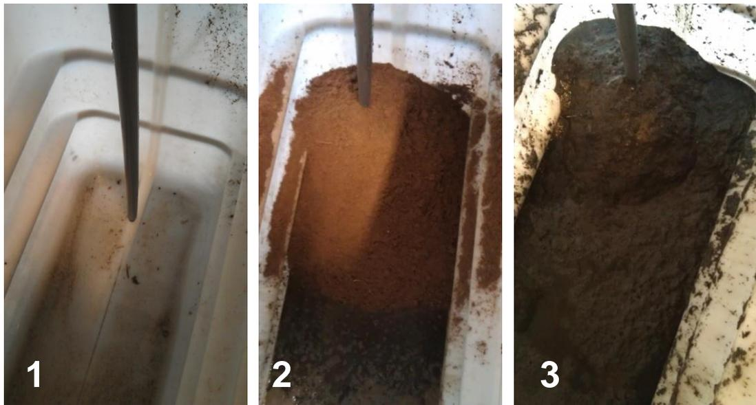
Figure 6. Photo 1 shows the LevelTec pressure sensor installed in the small scale slurry container used for the performance test. Photo 2 shows the LevelTec sensor covered by sand. Photo 3 show how the sand is placed around the LevelTec sensor after the slurry container was filled with slurry and emptied again. It is seen that the sand is still laying around the sensor.
