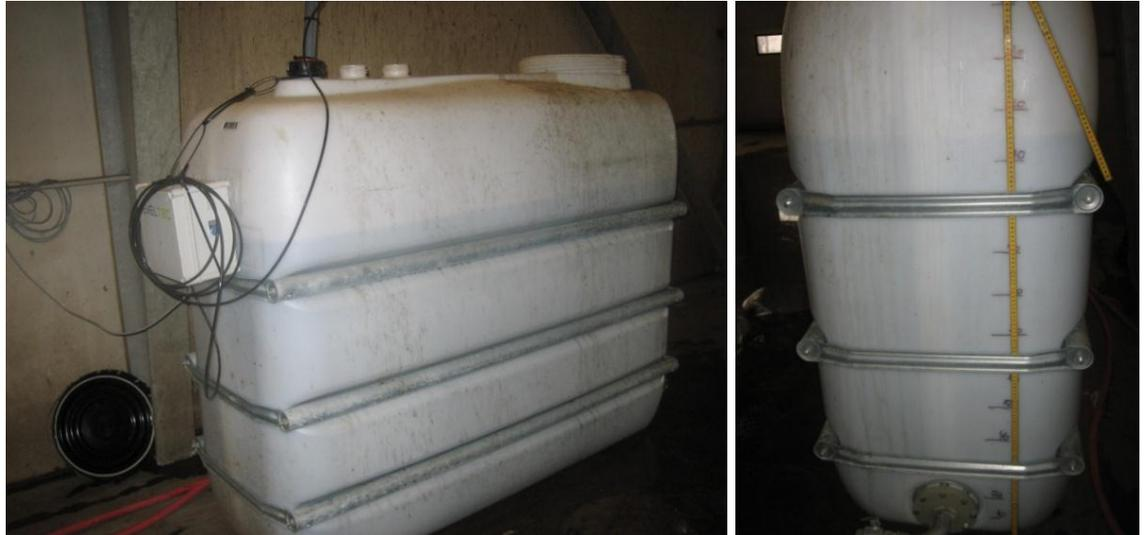
Figure 5. The small scale slurry container used for the performance test of LevelTec. On the left photo the LevelTec control unit is seen as a grey box installed on the end of the slurry container.
