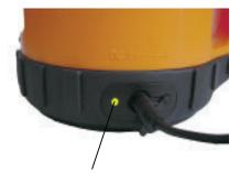
Note: Please charge the battery when the battery is empty (power LED on the instrument flash means the battery is empty), that could extend the battery use life.
