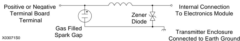
The spark gap is capable of conducting large amounts of current, but its response time is long compared to the rise time of most transients. The faster zener diode begins conducting during the rapidly rising portion of the transient, with the current flow through the zener diode limited by the inductor.
