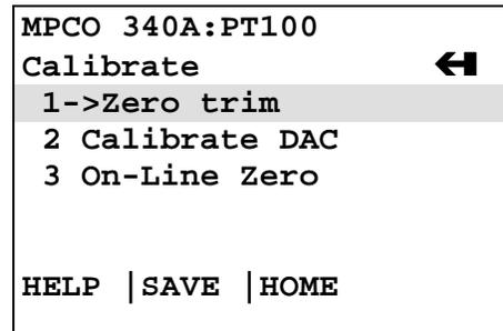
5. Press “1” on the keypad or press the RIGHT ARROW/SELECT key to access the Zero trim menu.
