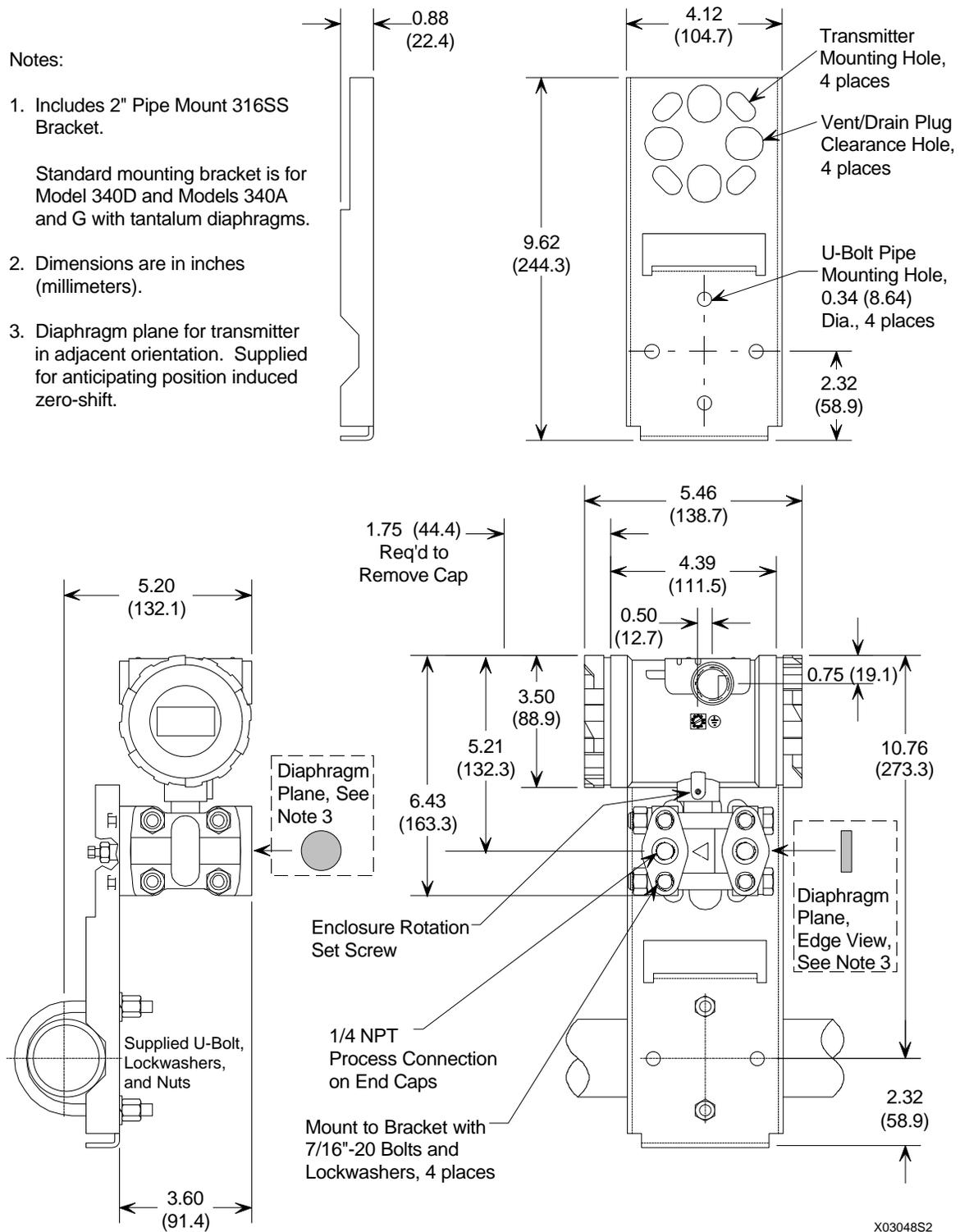
**FIGURE 4-10 2" Pipe Mount Bracket, Model 340D (See Note 1)**
