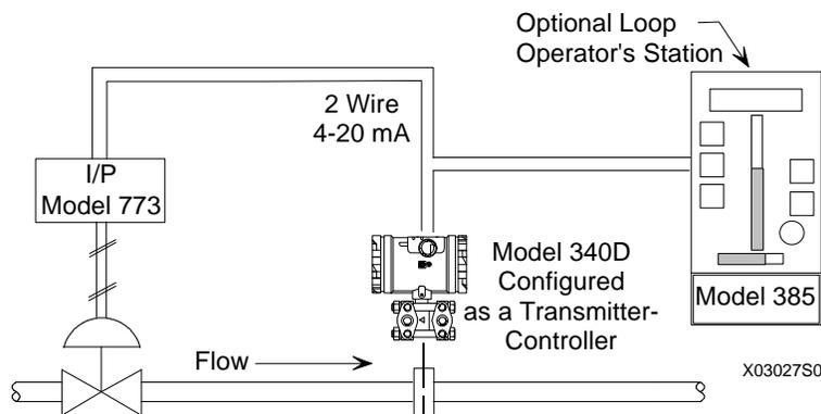
**FIGURE 1-5 Transmitter-Controller Application**
