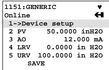
**Device setup** – provides access to the Device Setup menu. Configurable device parameters common to all HART-compatible devices can be accessed from this menu.
