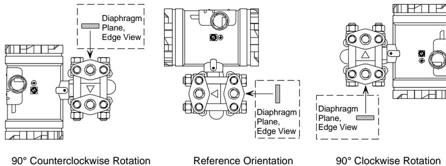
For example, in the drawing below, rotating the transmitter 90° either clockwise (terminal board end down) or counterclockwise (display end down) from the nameplate-on-top orientation will cause maximum zero shift because the diaphragm orientation changed from vertical to horizontal.
