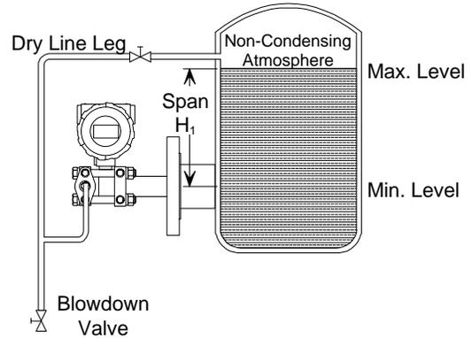
Closed Tank, Non-Condensing Atmosphere, Level Measurement
