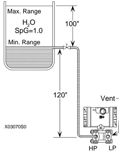
**FIGURE D-3 Elevation Calculation Example**
