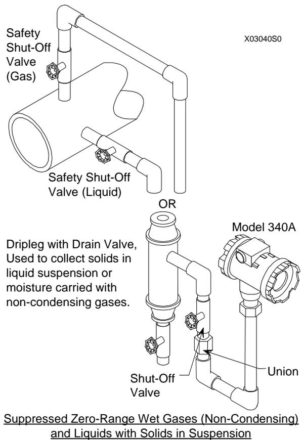
**FIGURE 4-3 Absolute or Gauge Pressure Measurement Piping**
