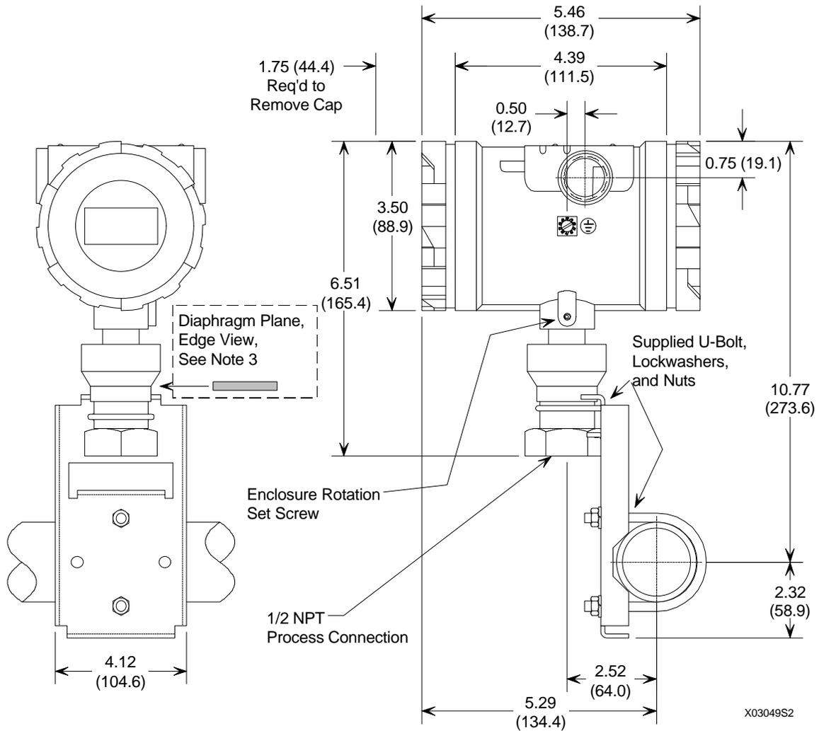
**FIGURE 4-11 Pipe Mount Bracket, Models 340A and G (See Note 1)**
