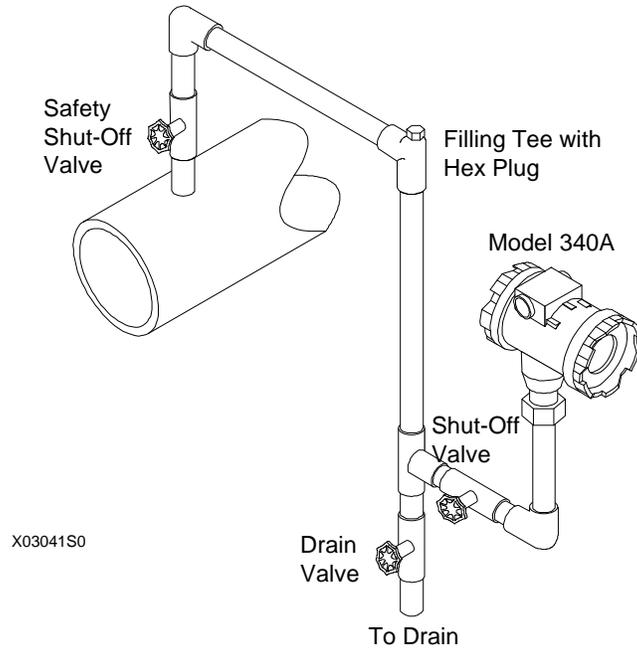
**FIGURE 4-4 Steam Service, Below the Line Mounting**
