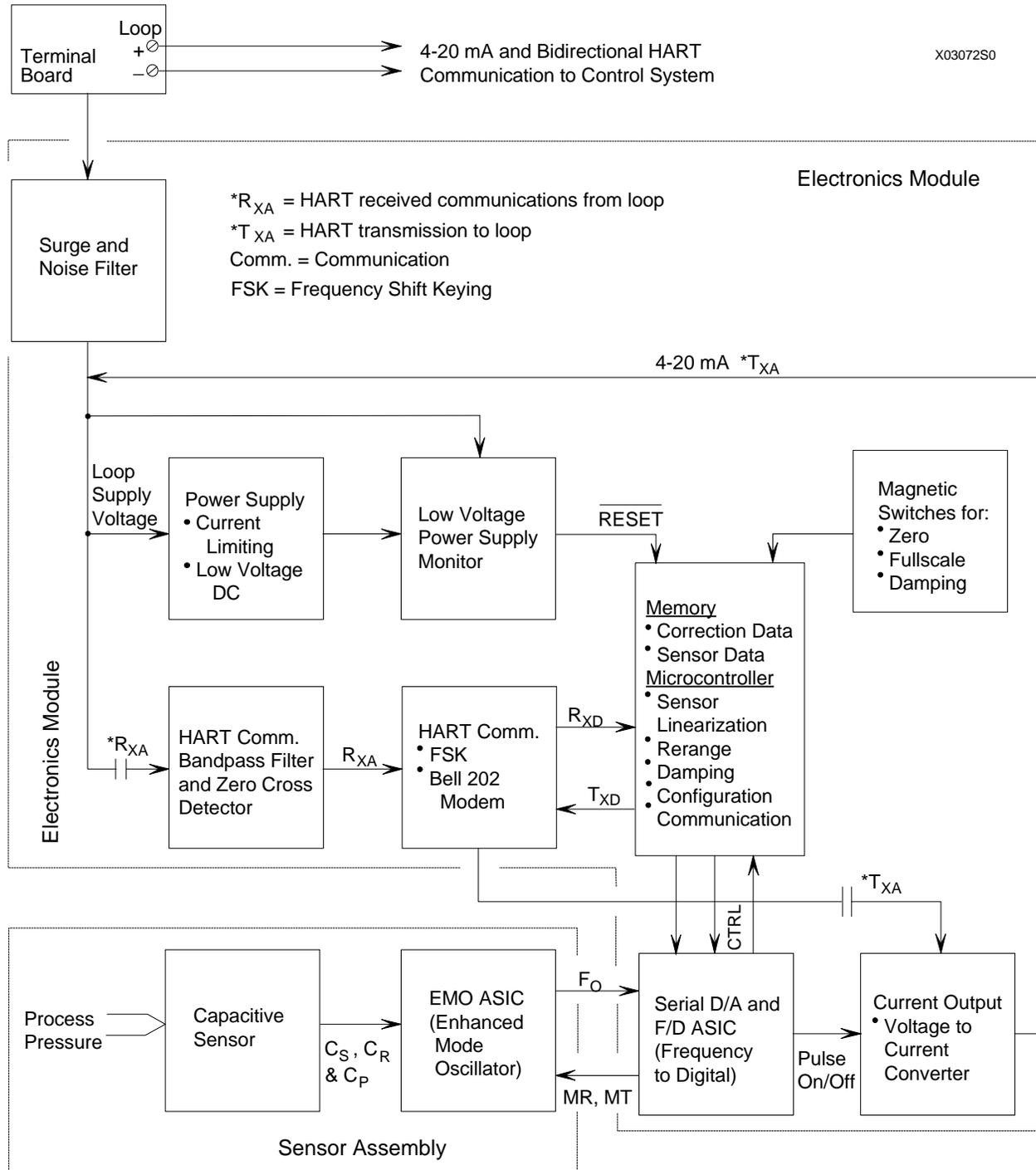
**FIGURE 8-1 Block Diagram, Electronics Module and Sensor Assembly**
