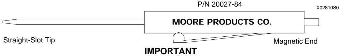
Use only the Moore magnetic screwdriver to actuate the magnetic switches. Other magnets can cause inconsistent behavior of one or more switches.
