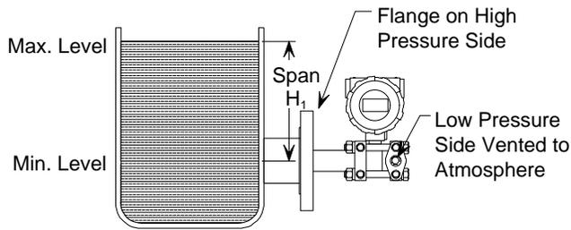
Open Tank, Level Measurement
