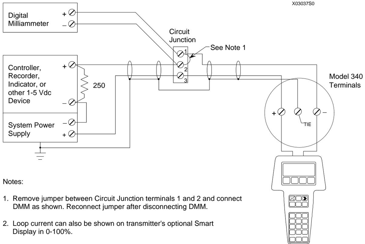
**FIGURE 3-2 Field Test Connections**
