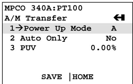
4. Use the UP or DOWN arrow key to select Yes (A/M change from Communicator only) or No (magnetic switches can be used to change mode), then press ENTER (F4) to confirm the selection or press ESC (F3) to return to the A/M Transfer menu without making a change.
