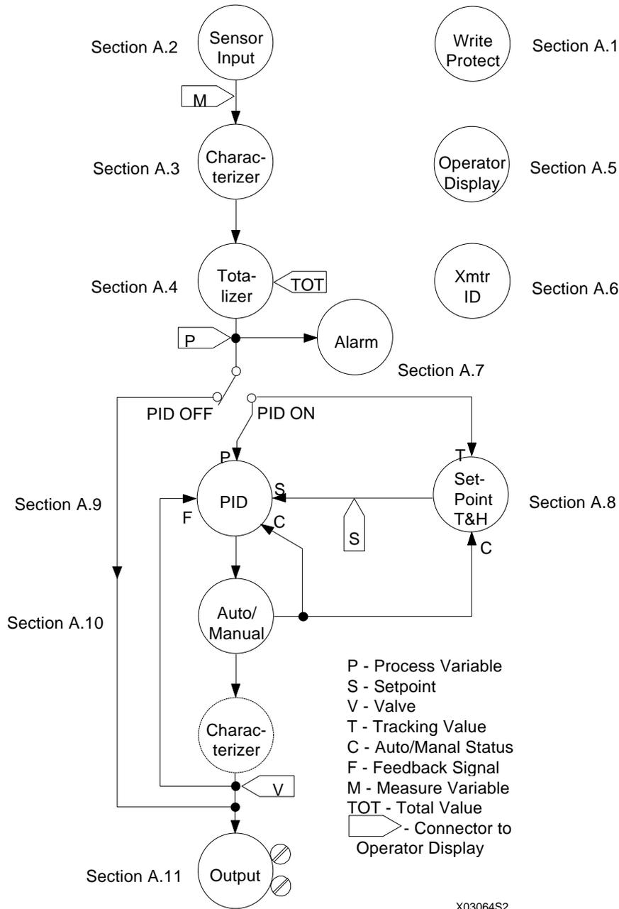
FIGURE A-1 Function Block Arrangement in Model 340 Transmitters
