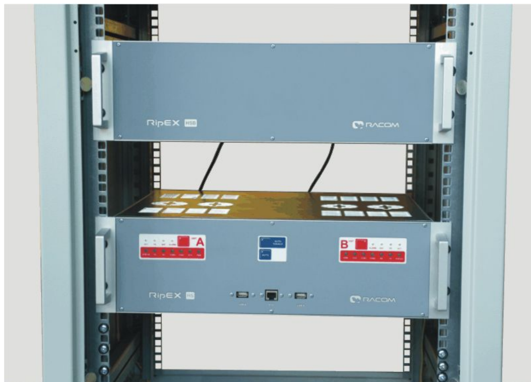
Fig. 5.3: RipeX-HS in 19" Rack Cabinet
