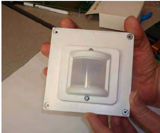
Figure 10. Assembled Flat 0.9" Lens Holder and Flat Lens
