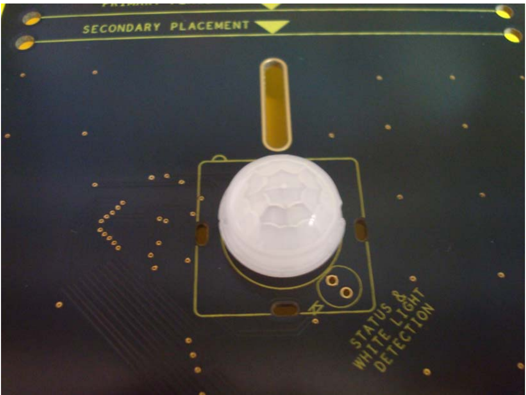
Figure 3. NCL-9(26) Lens and PIR Sensor Installed on the ZMOTION 20-Pin Development Board
