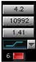
Top to bottom: Gain, Frequency, Q, In-out/Type
