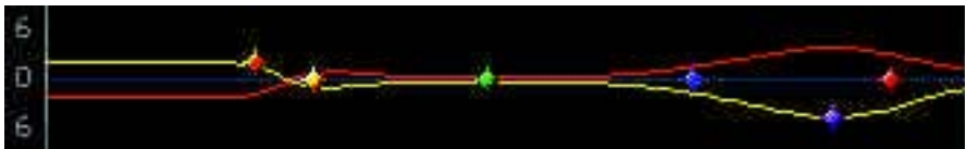
Separate (unlinked) equalization of L and R (or dual-mono)
