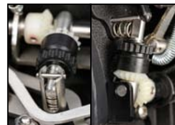
The spring-loaded sub and main command dial gear assembly
