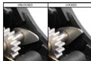
close-up shot of the port lock mechanism in the unlocked (left) and locked (right) positions.
