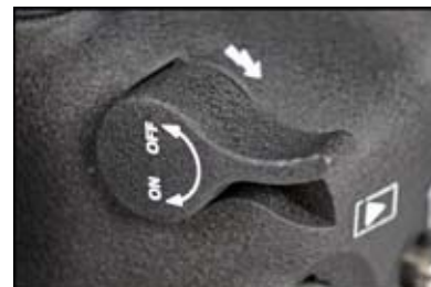
The two-way lever which controls the pop-up flash.
