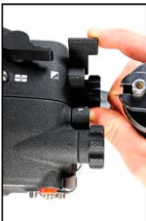
Holding the AE-L/AF-L lever depressed while keeping a finger firmly on the shutter release lever was easy.
