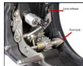
port lock and lens-release internal mechanism.
