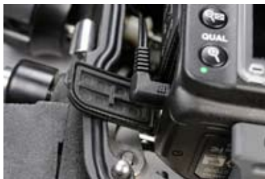
When the hydrophone is connected to the camera, the back plate o-ring is obstructed, so extra care must be taken when sealing the housing.
