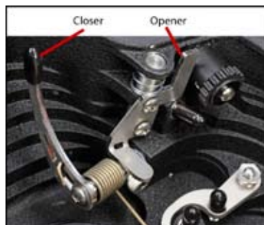
The inner-workings of the two-way flash lever
