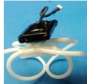
Rat Saddle Harness with Mounted 500 mAh External Battery
