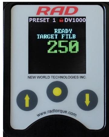
Figure 4.2.2-3: Main Screen in Locked Level
