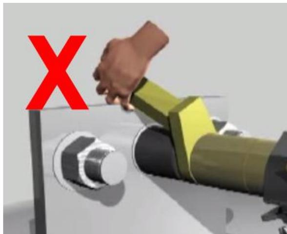
Figure 5.1.1-2: Incorrect Placement of Hand/Body Parts During Operation
