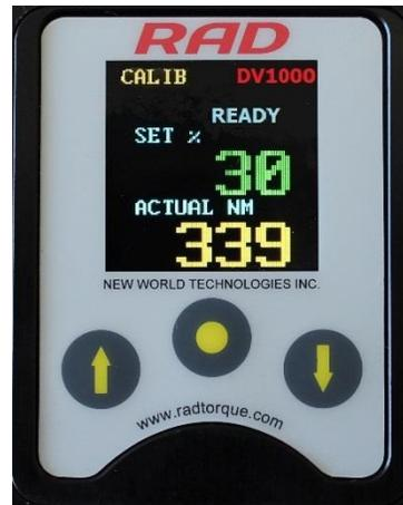
Figure 4.3.12-4: Calibration Screen – Actual Torque Highlighted
