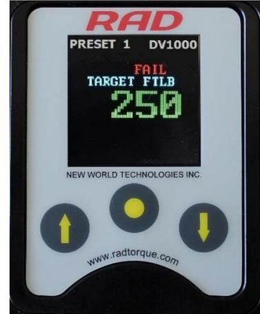
Figure 5.2-2: Failed Torque Cycle
