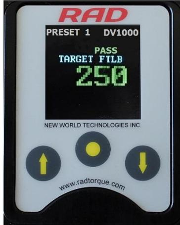
Figure 5.2-1: Passed Torque Cycle
