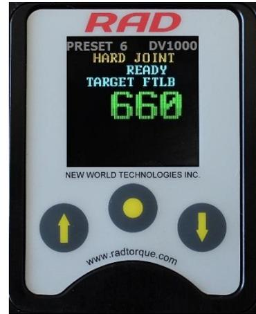
Figure 4.3.2-2: Main Screen – Hard Joint Mode
