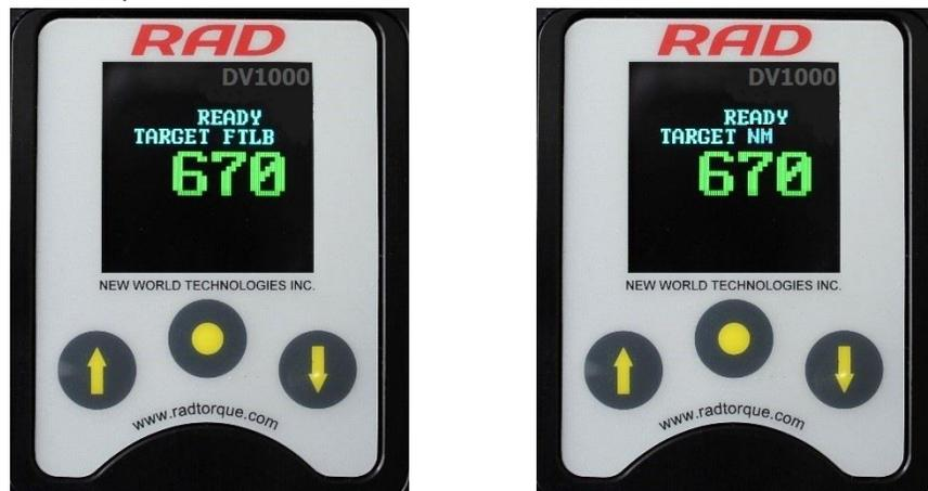
Figure 4.3.9-2: Different Units Displayed on the Main Screen
