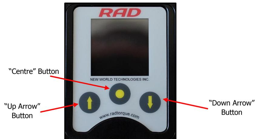
Figure 3.2-1: LCD Display Keypad
