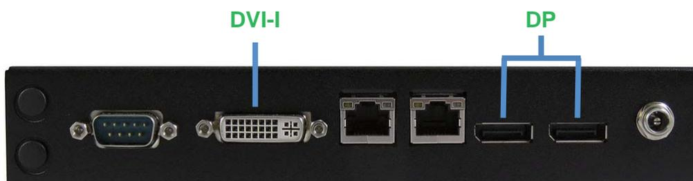
Figure 4 Connect the DVI-I / DP cable
