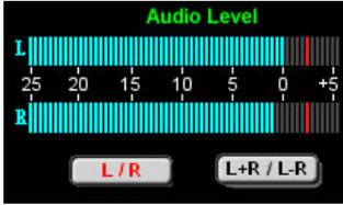
On the same indicator referred to previously, activating the **L+R/L-R** key, one can measure the addition and subtraction levels of the L and R channels. Therefore, on the upper VU meter, the mono component (L+R) of the signal transmitted will be indicated, and on the lower VU meter, the component of the L-R channel difference (which is the one that modulates the 38 KHz stereo subcarrier).
