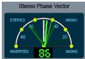
An important indicator of the quality of transmission sound is the Phase Vector, because it indicates the degree of **stereo sensation** the FM radio station transmits. This is linked, quite clearly, to the satisfaction index that the
