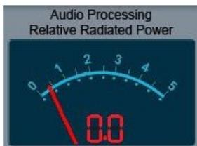
This important parameter is measured for the first time in FM radio transmissions. Its purpose is to inform the FM radio engineer of the effectiveness of the audio processing chain. This Effective Power with Processing (called RRP,
