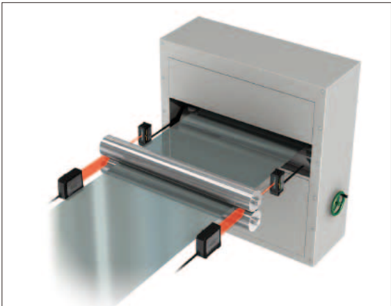
Gap measurement between rollers
