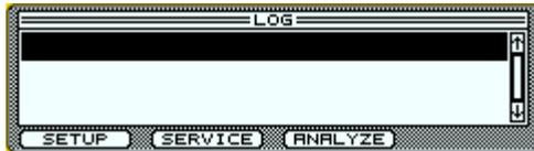
From the main menu (run display), press the down arrow to view the log of controller events.
