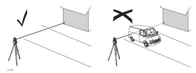
When measurements are being made using the red laser EDM, the results can be influenced by objects passing between the EDM and the intended target surface. This occurs because reflectorless measurements are made to the first surface returning sufficient energy to allow the measurement to take place. For example, if the intended target surface is the surface of a building, but a vehicle passes between the EDM and the target surface as the measurement is triggered from a field controller,
