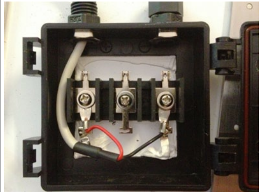
FIGURE 53: Solar panel's connectors box.
