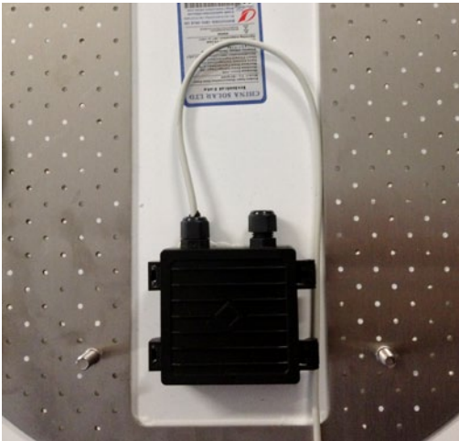
FIGURE 54: Leave the solar panel's wire slightly loose.
