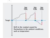
The isoCAL calibration and adjustment function will activate after a preset or configurable time period. Exceeding a preset or configurable temperature difference triggers a recalibration | re-adjustment.
