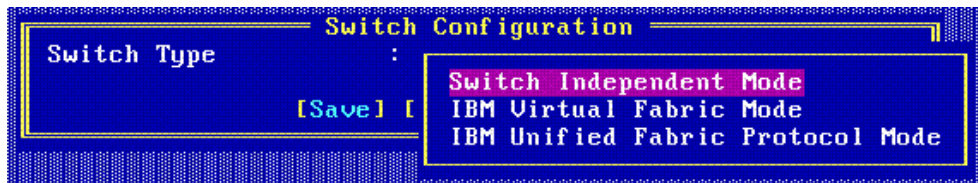
Figure 2-12 Switch Configuration Screen
