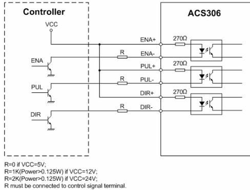
Figure 3-2: Connections to controller with common-anode outputs
