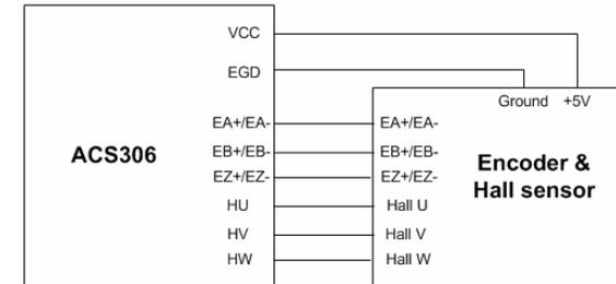
Figure 3-4: The ACS306 supplies the encoder directly
