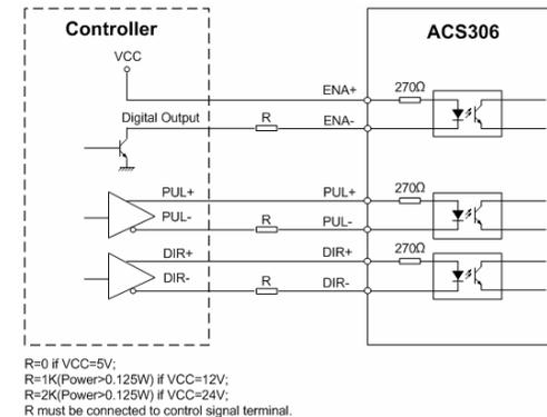
Figure 3-1: Connections to controller with differential outputs
