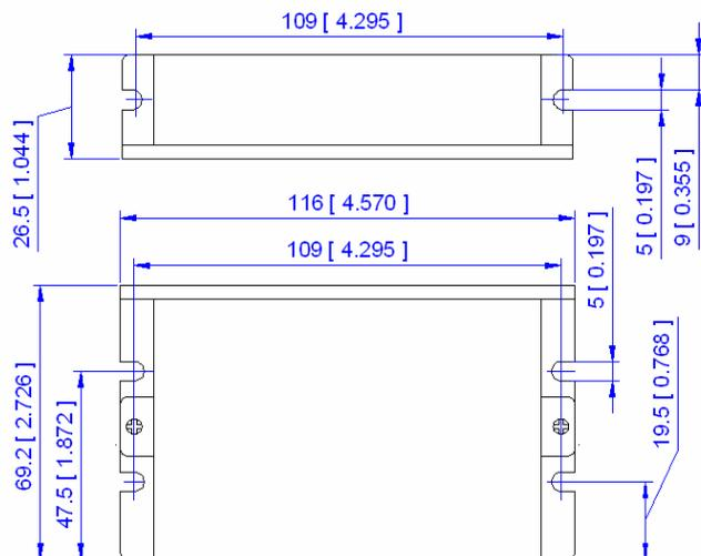
Figure 2-1: Mechanical specifications
