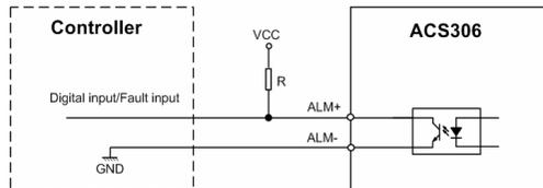
Figure 3-3: Connections to controller with alarm signal outputs
