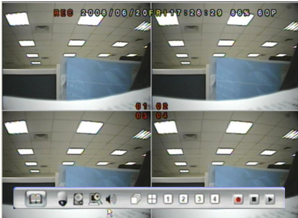
**NOTE : The pop-up menu can be activated by moving the mouse cruise to the bottom of the live viewing screen.**
