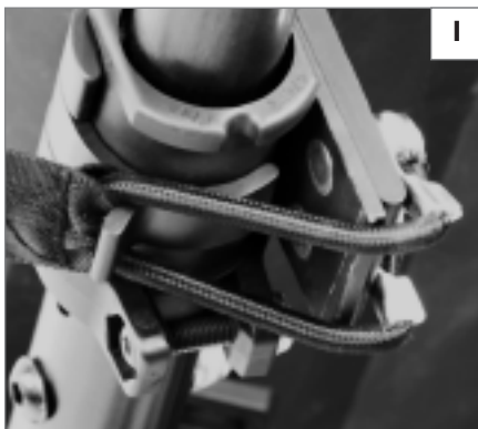
Check that the Snaptite Clamp is in locked position and secured with band.
