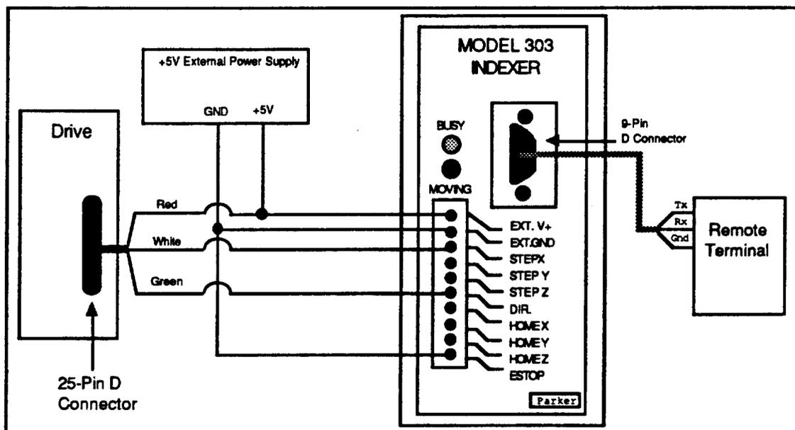
Figure 2-1. Basic System Wiring Diagram
