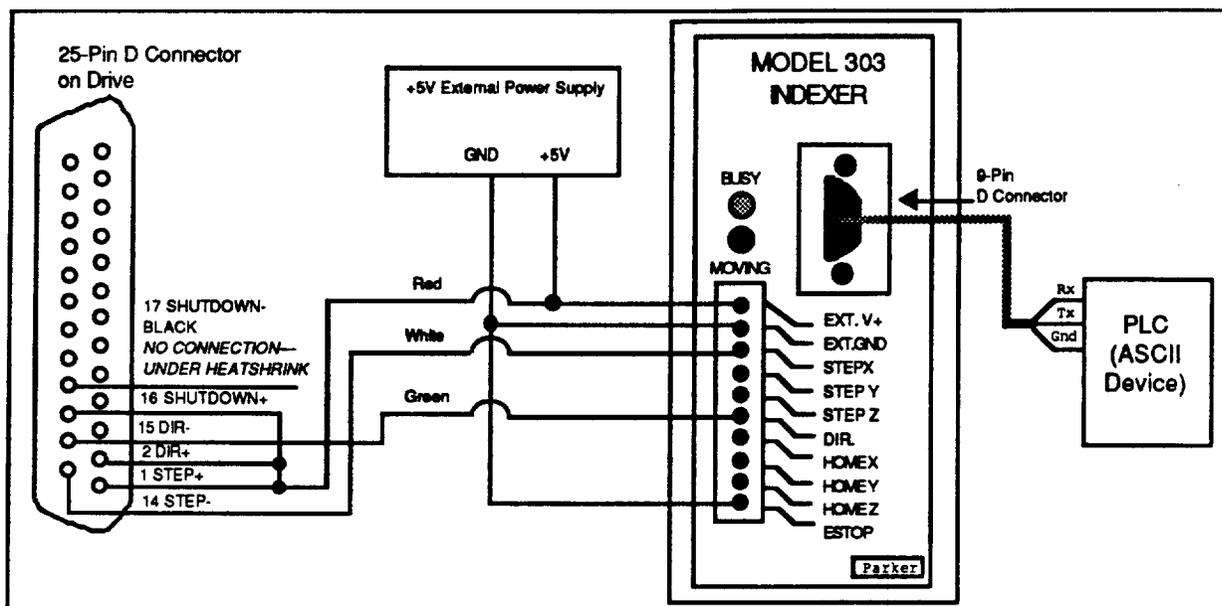
Figure 3-3. Complete Configuration
