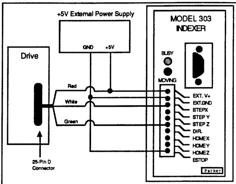
Figure 2-4. Model 303/Drive Connections
