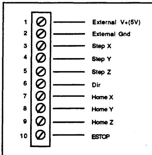
Figure 6-2. 10 Pin I/O Connector
