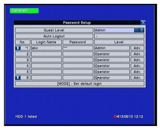
The Password Setup allows the administrator to add new users, delete existing ones, and/or modify the user's name, password, and/or level.
