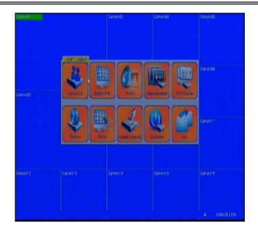
In Login/Logout display, press **Direction Control** button to highlight and select **Login** option, and then press **ENTER** to login the system. If the user wants to logout the system, just press **Direction Control** button to highlight and select **Logout** option, and then press **ENTER** button. Press **MENU/ESC** button to exit without making changes.
