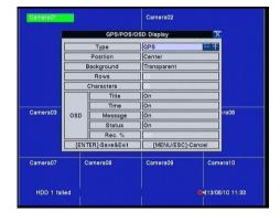
In the MONITOR mode, press the button to open GPS/POS/OSD Display setting. Please select the Type (GPS or POS), Position, Background, Rows, and number of Characters on the screen.
