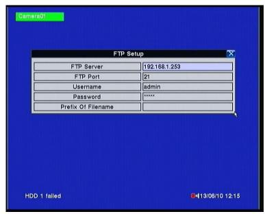
The FTP Setup allows the administrator to set FTP related parameters. When an event occurs and FTP is enabled for the action, the recorded video/audio for that event will be sent to the FTP server based on the parameters set here.
