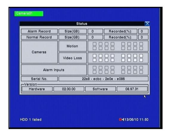
System info display includes Alarm Recording Status, Normal Recording Status, Camera Status, Alarm Input Status, Product Serial Number and Product Version Number. Press **MENU/ESC** to EXIT Status display to return to Menu display.
