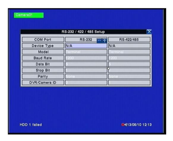
The RS-232/422/485 Setup allows the administrator to setup RS-232 control port, and RS422 or RS-485 control port. Please refer to the manuals for the connected devices - PTZ cameras or keyboard controllers – to set these items in RS-232/422/485 Setup.
