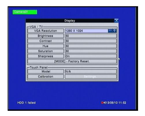
There are 5 items which can be adjusted, including Resolution (1280x1024, 1024x768, 800x600, 640x480), Brightness, Contrast, Hue, and Saturation. The operations are as below:
