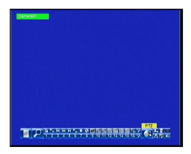
The system supports X2/X4 Digital Zoom function. To use this function, press button in full screen display to enter Digital Zoom mode.
