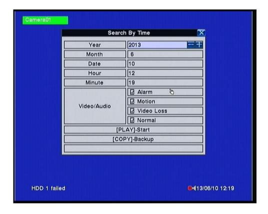
The Status area will show the 'Recorded from' time based on the selected Video/Audio before searching - alarm partition if any of Alarm, Motion, or Video Loss, is checked, and normal partition if Normal is checked.
