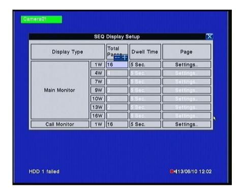
The SEQ Display Setup allows the administrator to define the display pages in SEQ Display for main monitor and call monitor. There are up to 7 display types - 1-Window, 4-Window, 7-Window, 9-Window, 10-Window, 13-Window and 16-Window -for main monitor, and 1 display type for call monitor.
