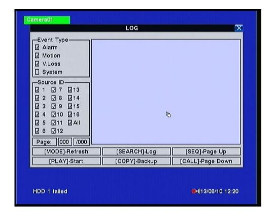
There are four types of event logs including Alarm, Motion, Video Loss and System. And up to 3000 most recent event logs can be stored in the system.
