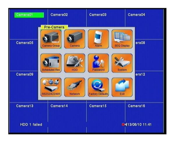
If the user wants to reset all the settings to factory default values, you may press **Direction Control** to change the highlighted option to **Factory Defaults**, and then press **ENTER**. A confirmation dialog will be shown, press **ENTER** again to make the changes, MENU/ **ESC** to not do it.
