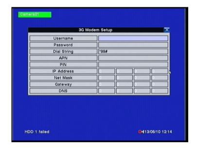
3G modem settings allow the administrator to set the modem parameters of 3G USB dongle
