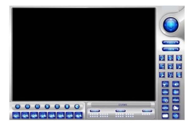
The video images can be displayed in several types of split-window screens, including 1/4/9/16-Window for single DVR and 25/36/49/64 for multiple DVRs. And the focus window is surrounded by a frame border. In addition to the video windows, there are different icons on the lower corner and the right corner of the screen for status display and control.
