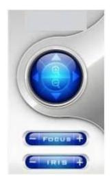
**PTZ control panel**. If the camera in the focus window is a PTZ camera, these buttons in the PTZ control panel can be used for PTZ control. The operations include Tilt Up/Down, Pan Left/Right, Zoom In/Out, Focus Near, Focus Far, Iris – (darker), Iris + (brighter).
