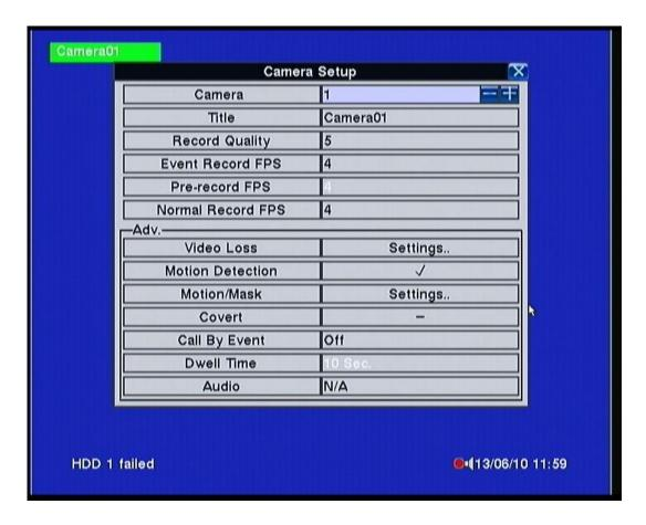
The Camera Setup allows the administrator to define the attributes for each camera. There are up to 16 or 9 cameras which can be connected to the system.
