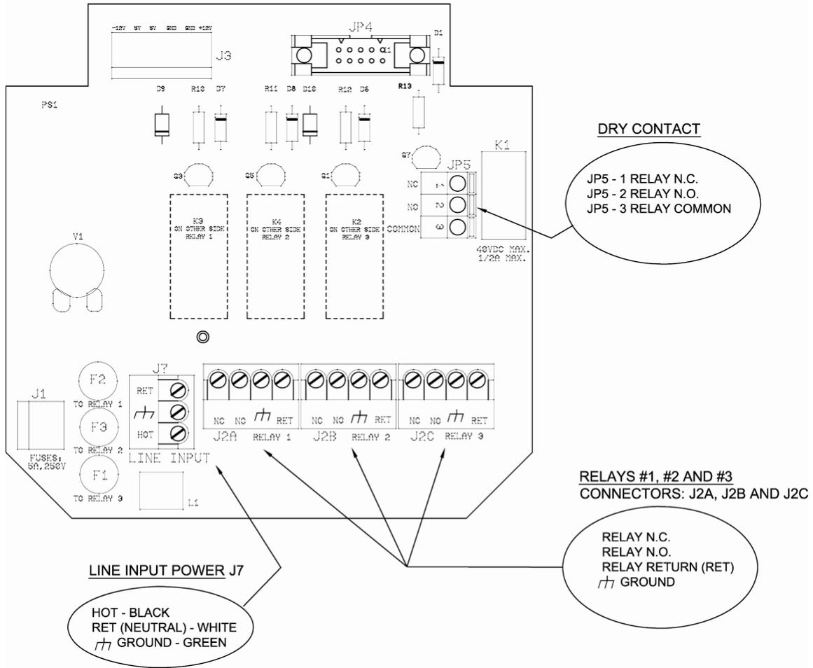
Conduit units are factory predrilled with easily accessible terminals for hard wiring. See Relay Board, Diagram 4, page 29, and Electrical Wiring section in this manual, page 7.
