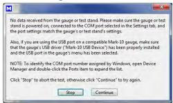
This message appears when communication has not been achieved between the instrument and MESURgauge, due to a number of possible causes:
