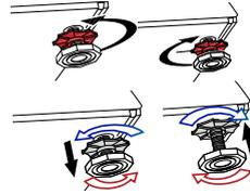
**WARNING:** Do not use any tools to loosen the lock nuts. Otherwise, they will get damaged.
