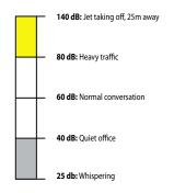
Some examples of typical noise levels. A quiet office may range from 40-50 dB, while a road drill can produce 100-110 dB.
